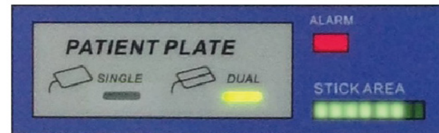
Neutral electrode recognition & contact area monitoring and display
